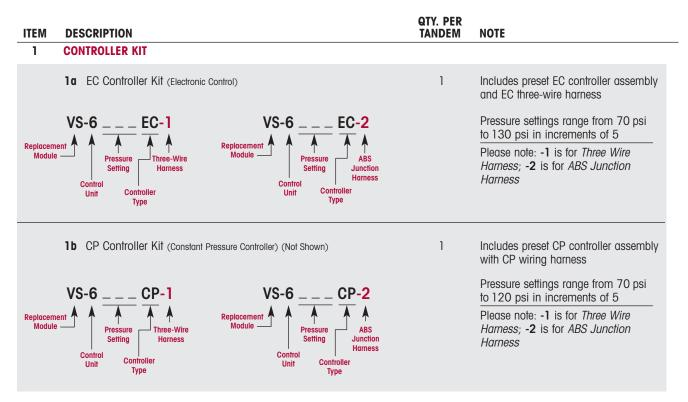
Example: EC Controller Kit Part Number VS-6100-EC-2 is 100 psi with ABS Junction Harness CP Controller Kit Part Number VS-6100-CP-1 is 100 psi with Three-Wire Harness
